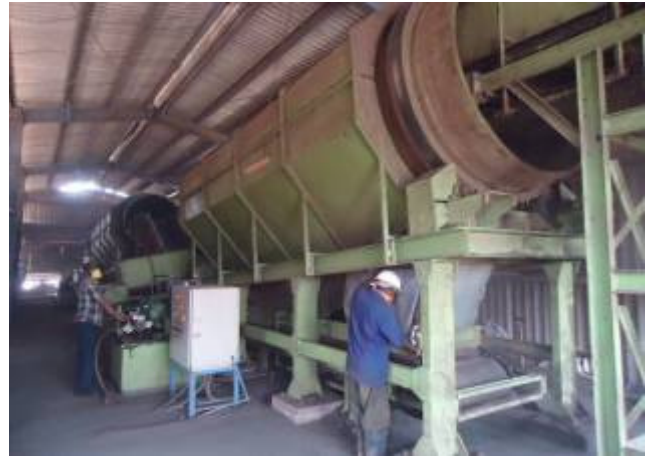
Screening through 35mm & 16mm Trammels
