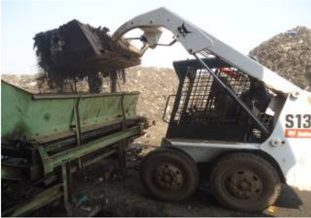
Fermented MTL Feeding to 35mm Trammel
